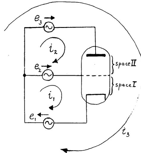
Fig. 2.—Basic triode circuit treating the valve as a passive circuit element.  $i_1$ ,  $i_2$  and  $i_3$  are mesh currents, and  $e_1$ ,  $e_2$  and  $e_3$  are ideal zero impedance small-signal generators.
