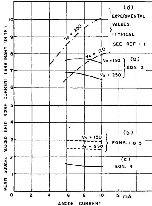
Fig. 1.—Values of induced grid noise : (a) Calculated on the theory of references 3, 4 and 5; (b) Calculated on the theory of reference 1 with theoretical values of  $c_i$ ; (c) Calculated on the theory of reference 2; (d) Typical experimental values. (Reference 1.)
